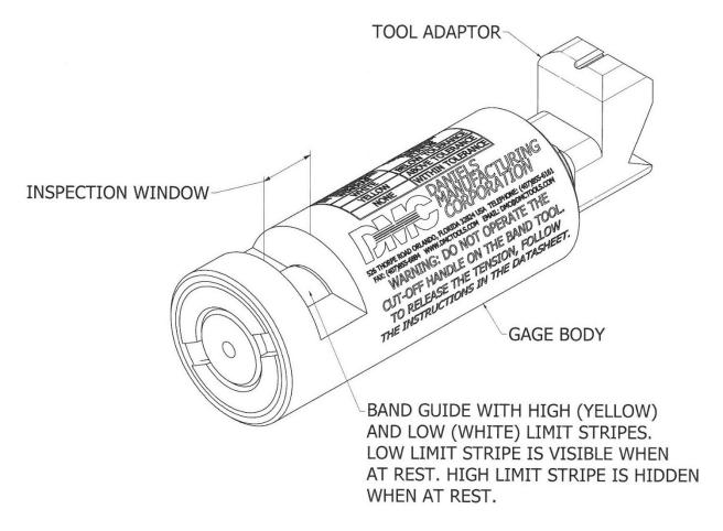
Warning: Keep the DBS-CG8 in a clean, dry place when not in use. Keep the inspection window free from dust and debris.
