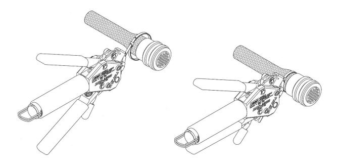
Apply an adequate amount of pressure in line with the cable as it enters the backshell to allow the 1/8 inch space to be reduced to zero. The tool is then activated to the preset tension, and terminated/cut using the procedure described in section 1.0 of this guide.
