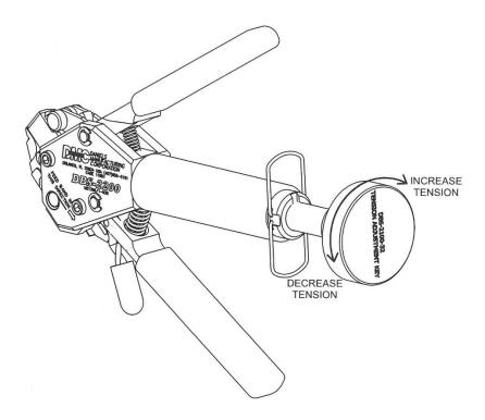
Step 4: Verify the tension applied to the band is within the specified tolerance
