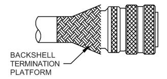
The braid is pushed into position over the backshell termination platform. Care must be taken to make sure the weave is uniform and no large "windows" are present. A shield termination band is loaded into the tool. If the band is uncurled it must be double looped through the buckle before termination. The band is then slid into a position of alignment with the backshell termination platform.
