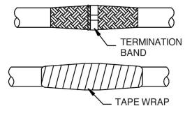
Heat-shrinkable tape is then applied over the splice. When a jacketed cable is used, be sure the tape extends onto the jacket in both directions.
