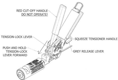
NOTE: <u>DO NOT ATTEMPT TO CUT THE BAND</u>. DAMAGE TO THE TOOL AND/OR GAGE MAY OCCUR.
